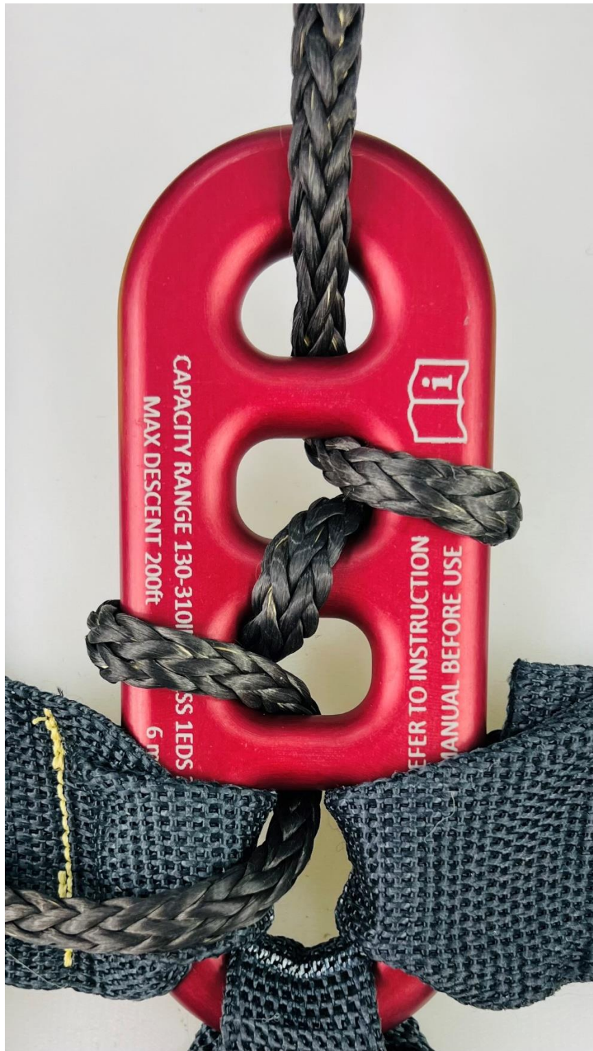
Level 2 Line Configuration, 200 to 280 lbs. Photo 2
