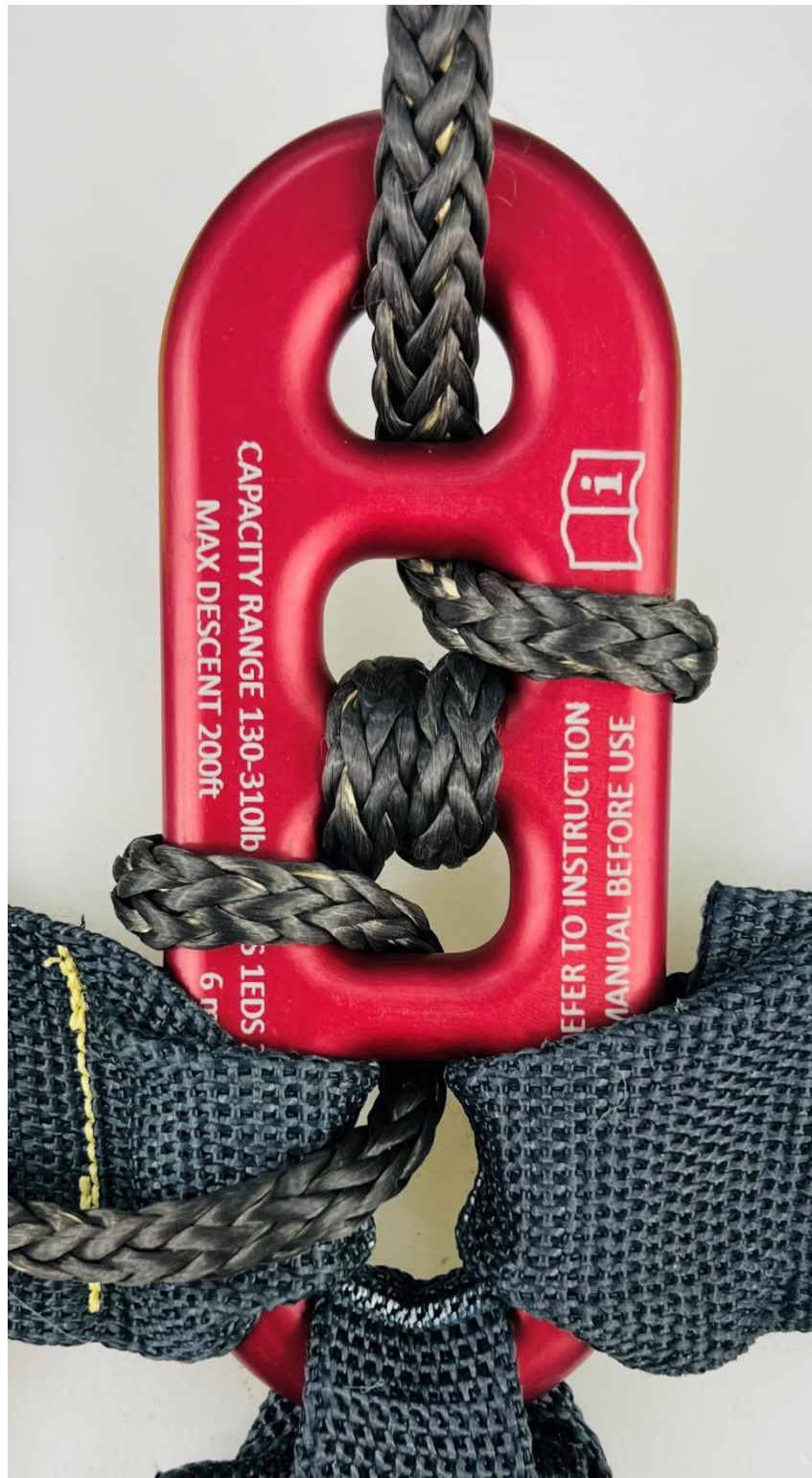
Level 3 Line Configuration, 280 to 310 lbs. Photo 3
