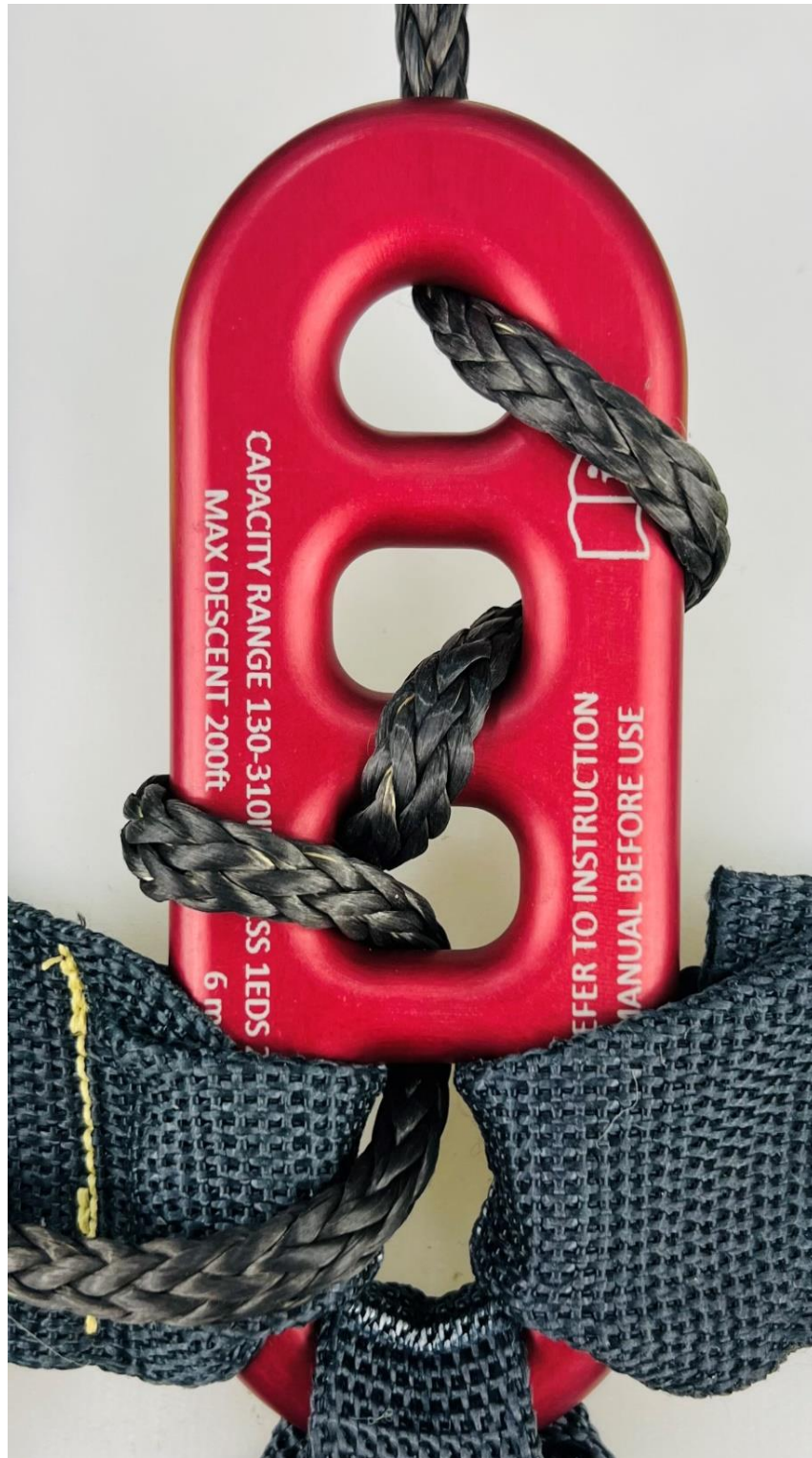
Level 1 Line Configuration, 130 to 200 lbs. Photo 1
